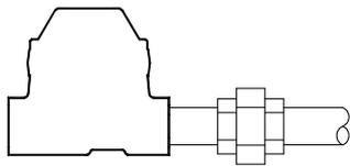
Fig.7 With union for easy dismantling
