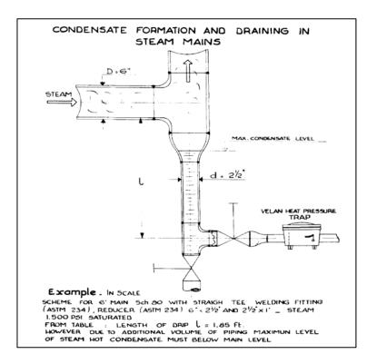
Drip legs should be installed roughly every 300 feet and never more than 500 feet. In a supervised warm up drip legs should be minimum of 10 inches long. Drip legs on automatic warm up systems should be a minimum of 28 inches long. As a rule of thumb drip leg length should be 1.5 times the diameter of the steam main. Drip leg diameter should match steam mains up to 4 inches. Above 4 inches the drip leg should be at least half the diameter of the steam main.
