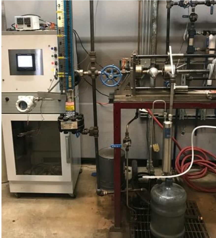
Test rig with condenser on steam trap discharge
