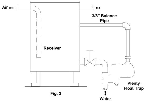
Fig 4 shows how this oil can be removed from a receiver. The water connection to the trap is taken from the bottom of the receiver where cleanest water is.,A drain valve is fitted at a higher level from which the oil and scum can be run at intervals.
