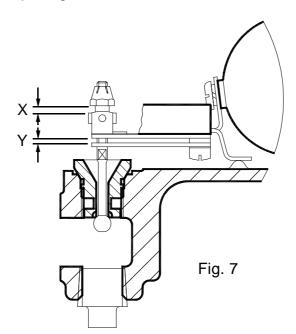
The standard factory setting is calculated at an ambient temperature of 65 F (18.3 C). If setting takes place at an alternative ambient temperature the clearance must comply with the setting table shown on next page.
