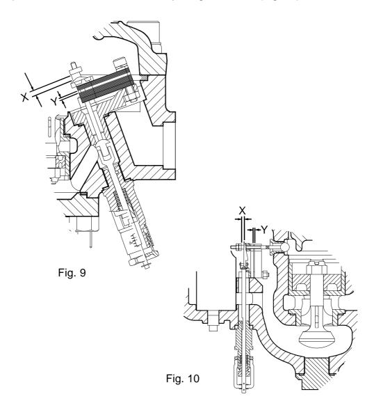
The standard is made at a temperature of  $65^{\circ}F$  ( $18^{\circ}C$ ) and will allow the valve to commence opening at  $15^{\circ}F$  ( $8^{\circ}C$ ) approx below saturation with full discharge, as shown in the capacity diagrams for each model, around  $40^{\circ}F$  ( $22^{\circ}C$ ) sub-cooling. When the ambient temperature changes, an alternative setting as shown in the table below should be used.
